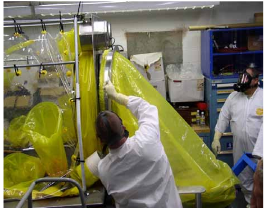
Trainee learning to connect parent drum to glove bag.
